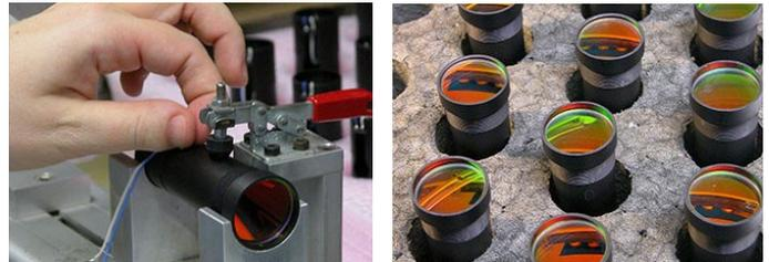
*The manufacture of all red-dot sights requires dust-free areas when assembling optics. Precise placement of adjustment turrets is necessary, as is that of the diode/emitter to ensure accuracy. While MRDS sights use smaller emitters to project the dot, they need to be just as rugged as a full-size dot sight in order to safely withstand the forces of a reciprocating slide.*
